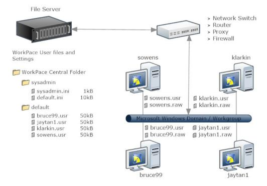
Illustration of the Network installation method of WorkPace: Four users are logged onto their computers and have their WorkPace User files updated onto the network File Server. Global settings for their User Group 'default' may be modified centrally by editing the file 'default.ini' within the directory 'sysadmin'.
